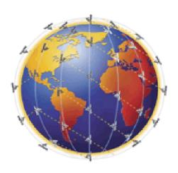
km). They circle the earth once every 100m minutes traveling at a rage of 16,832 mph. This constellation ensures that every rgion on the globe is covered by at least one satellite at all times
